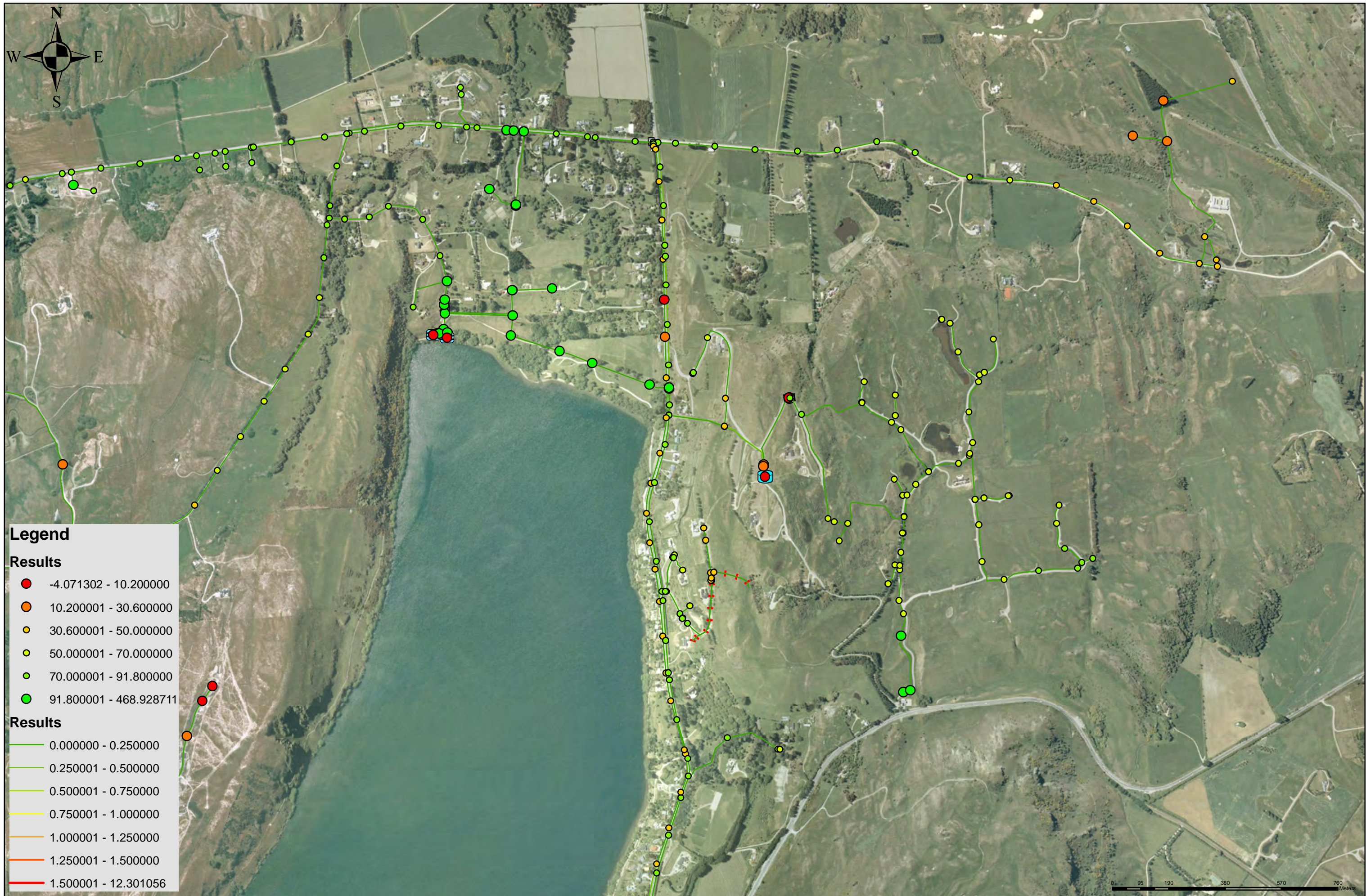
QLDC Water Supply - Arrowtown Retirement Village - Option 2, 200 mm Main, Normal Peak Day Demand Results
