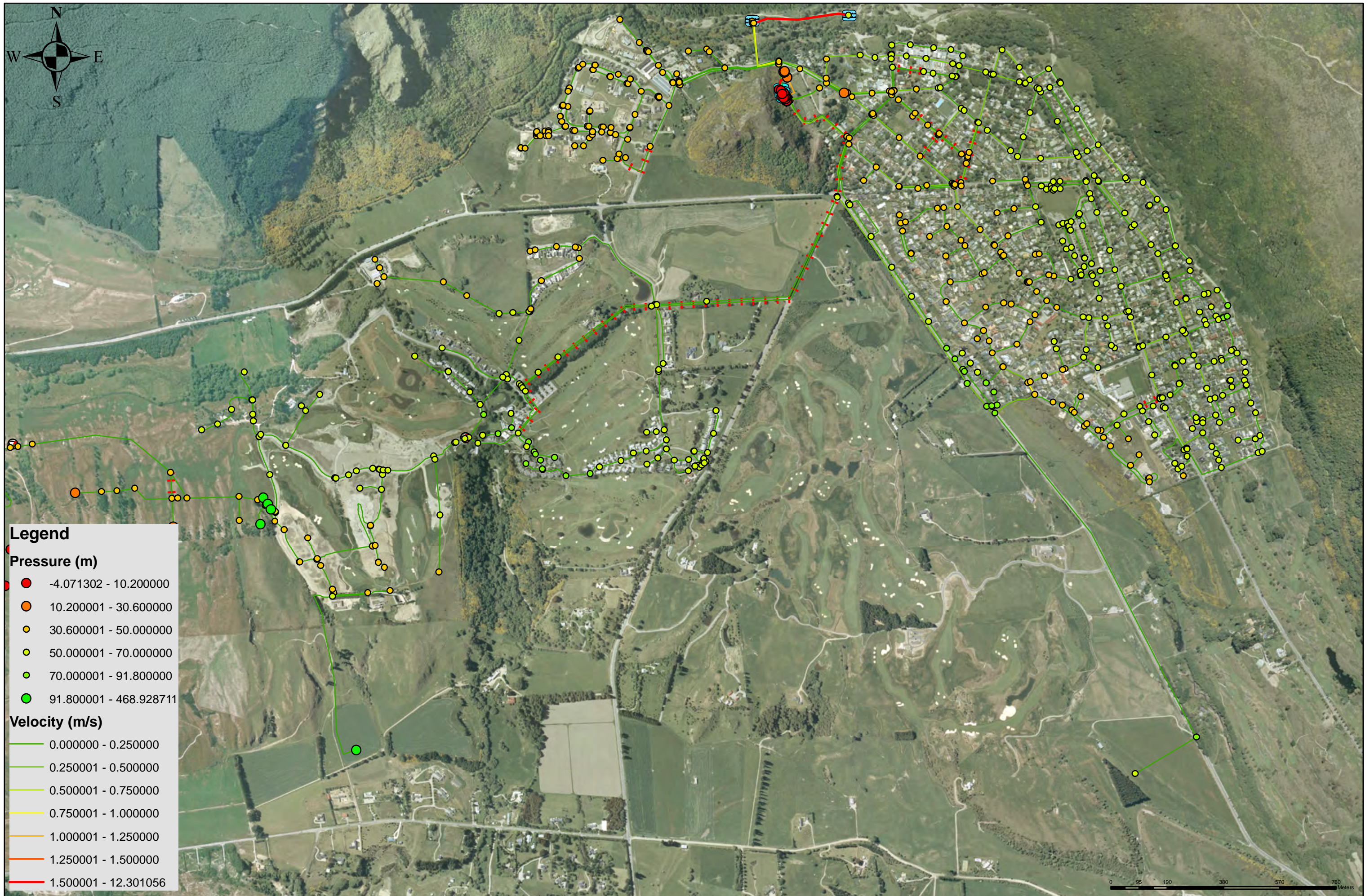
QLDC Water Supply - Arrowtown Retirement Village - Option 1, 200 mm Main, Peak Day Normal Demand Results
